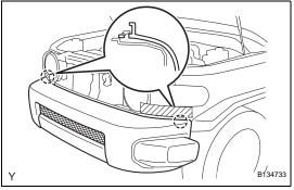
(b) Engage the 2 claws and install the front bumper cover.
