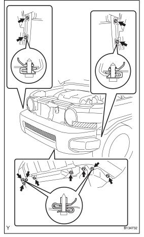
(c) Tighten the 8 screws and the 4 bolts.
